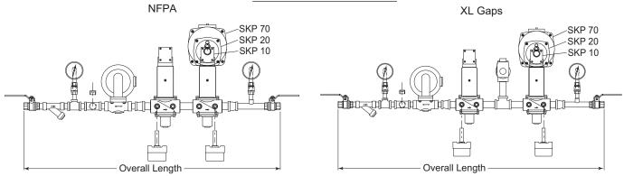
When using the Siemens SKP20 and SKP70 actuators for pressure regulating and ratio regulating functions, the sensing piping is not included. For proper operation, the sensing pipe should be at least 1/4" I.D. and connected a minimum of 5 pipe diameters downstream in a non-turbulent area.
